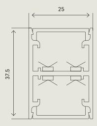
Smallest radius is 300mm, can be both surface mounted and suspended.
